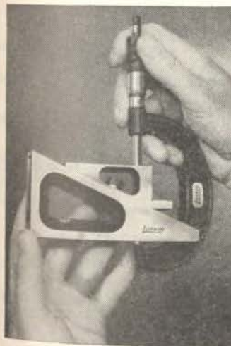
Gage Being Set to Micrometer Accuracy
