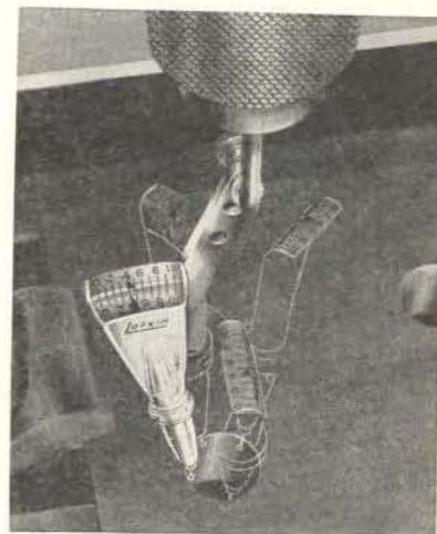
Indicating Hole in Jig Bore, Milling Machine or Drill Press
